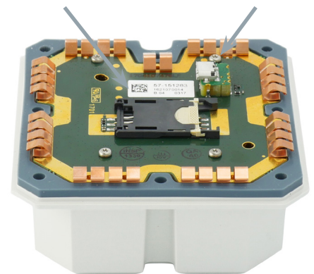
Cellular SIM Card Holder Micro USB Connector Short cable included
