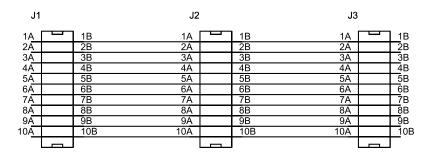
Figure 2-24: SAILOR 6209 Accessory Connection Box, diagram
