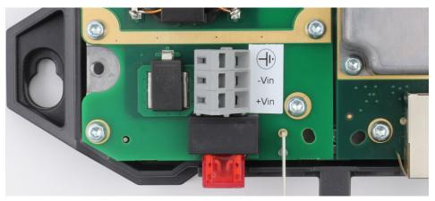
Figure 2-13: Transceiver Unit, connect power cables
