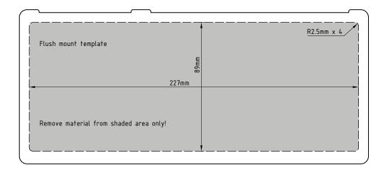
Figure 2-6: Control Unit, Cutout for flush mount
