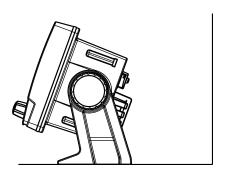
Figure 2-3: Control Unit, Mounting with the mounting bracket
