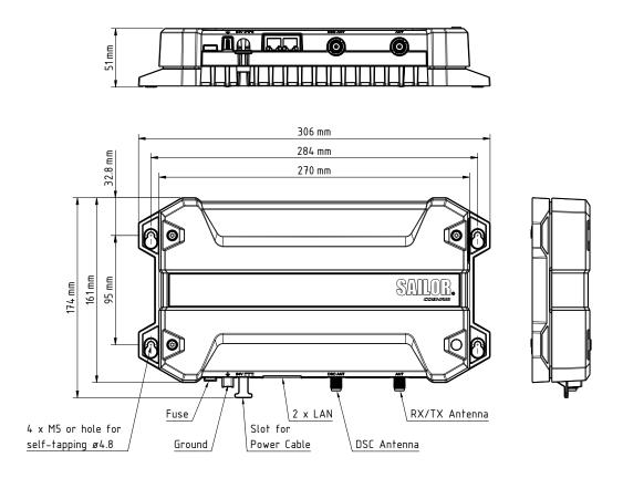
Figure 2-8: Transceiver Unit, dimensions
