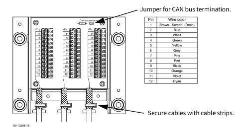
Figure 2-20: SAILOR 6208 Control Unit Connection Box for parallel handsets, wiring
