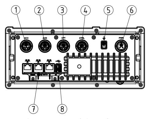
Figure 2-10: SAILOR 7224 Control Unit, rear panel connectors
