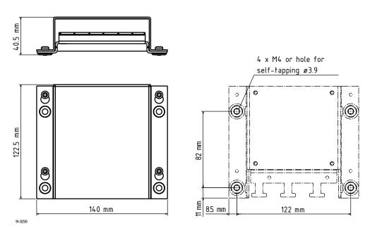
Figure 2-16: SAILOR 6207 Connection Box for parallel handsets, mounting
