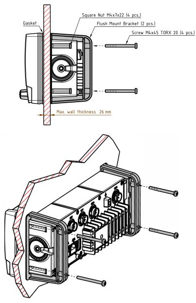
Figure 2-7: Control Unit, Flush mount
