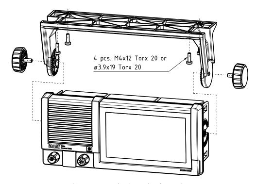
Figure 2-2: Control Unit, Overhead mounting
