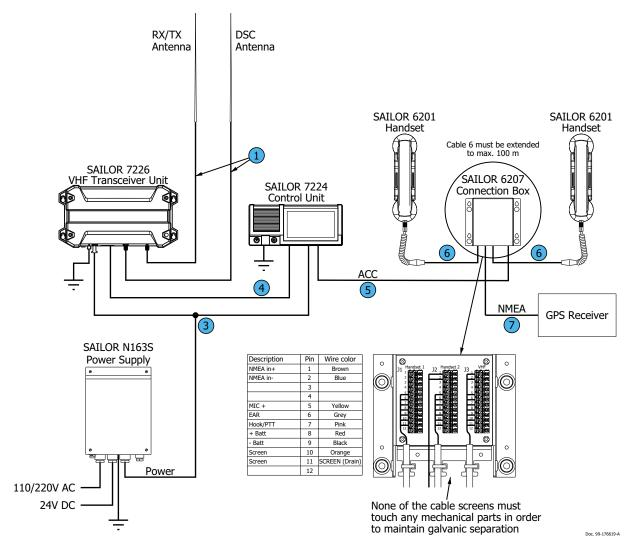
Figure C-4: System configurations, 2 SAILOR 6201 Handsets and a GNSS
