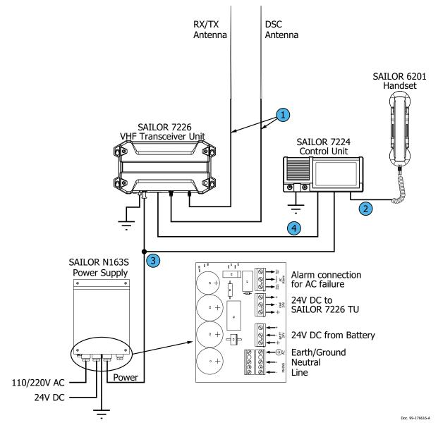
Figure C-1: System configuration, SAILOR N163S Power Supply
