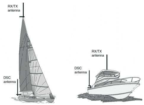
Figure 2-15: Antenna positioning, 2/2
