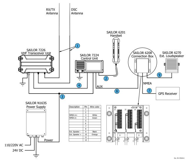
Figure C-3: System configuration, GNSS and SAILOR 6270 External loudspeaker
