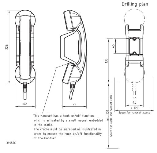
Figure 2-9: SAILOR 6201 Handset with cradle, dimensions for mounting.
