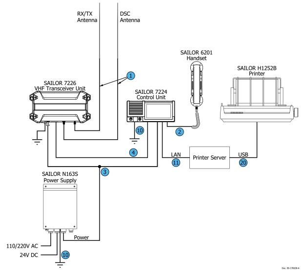
Figure C-15: System configuration: Installation of a printer
