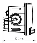
Figure 2-5: SAILOR 7224 Control Unit Dimensions for flush mount
