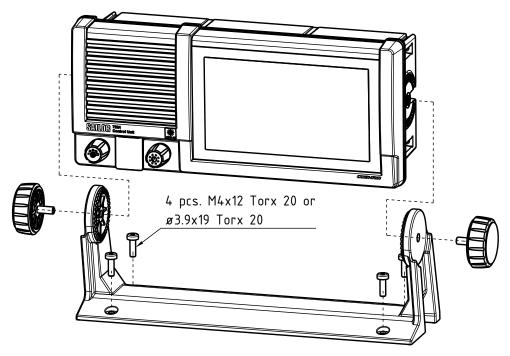
Figure 2-1: Control Unit, Desktop mounting 1/2
