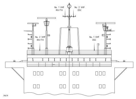
Figure 2-14: Antenna positioning 1/2
