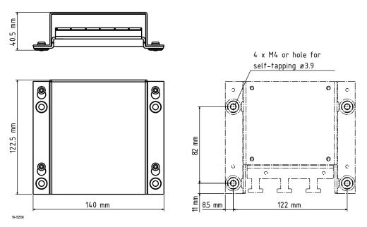
Figure 2-19: SAILOR 6208 Control Unit Connection Box, mounting
