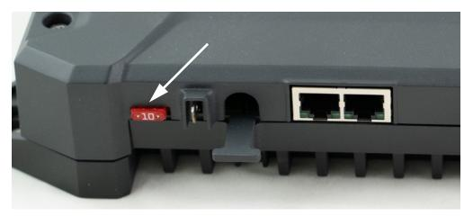
Figure 5-1: Fuse in Transceiver Unit
